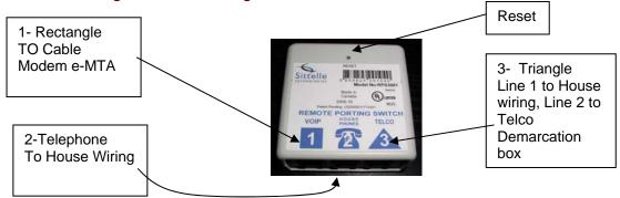
The Remote Porting Switch requires no external power connection. Each unit is independent and powered by the telephone line providing service.
